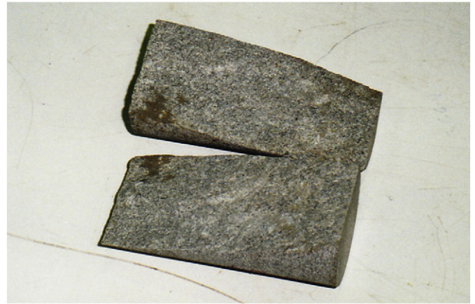
Fig. 1. Photo of the fractured granite specimen used for the experimental work.
