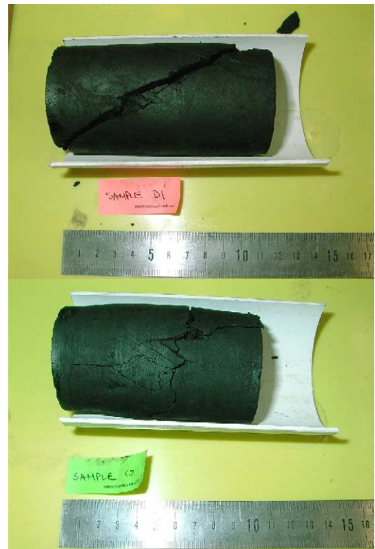
Fig. 9. Typical failed triaxial specimens.
