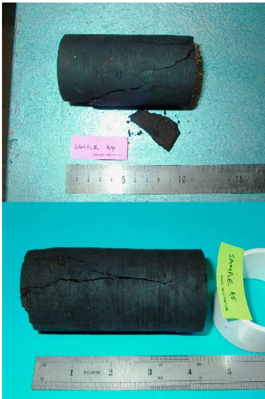
Fig. 6. Typical failed uniaxial specimens.
